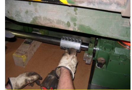
Vibrator to vibrator alignment shaft with couplings
