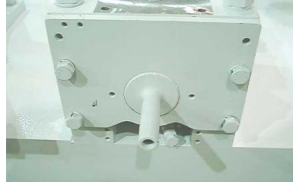
Motor alignment Hydrostatic drive
